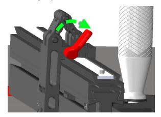
4. The Flip Stop Assembly is now installed and positioned for your first cut. Reposition the Flip Stop Assembly as needed for future cuts by releasing the red, flip stop clamp as described above, then securing it again at the new location.
