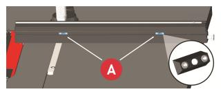
Using the spare, knurled Thumbscrew provided with your miter gauge, fix the wedges in place by tightening the set screws located on either side of the center hole in the Sliding Wedges.
