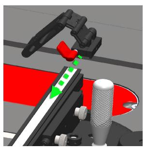
2. Continue to slide the Flip Stop Assembly along the top of the Fence Assembly extrusion to the desired distance from the blade.
