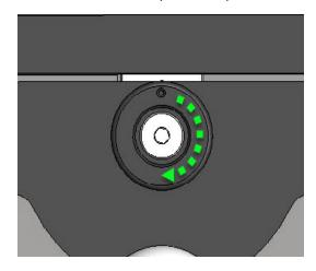
3. When you are satisfied with the adjustment, retighten the silver screw you loosened in step 1 using the included 3mm hex wrench. It is important that this screw is tight.
