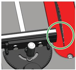
2. Adjust the Fence Assembly to the left or right as needed, then tighten the Thumbscrews on the back side of the miter gauge body to secure the fence from moving during cutting operations.
