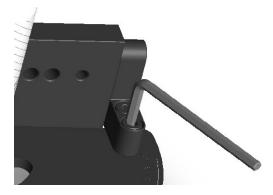
5. Use a precision square against the side of the miter bar without expansion discs to square the Vertical Faceplate as you re-tighten the four Socket-Head Bolts you loosened in step 4. Use the included 4mm hex wrench to tighten the bolts.
