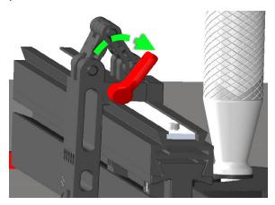
Insert a spare Sliding Wedge into the slot on the front of the Fence Assembly and position it behind the flip stop. Align the center hole of the Sliding Wedge (highlighted in blue) with the center hole on the front of the flip stop.
