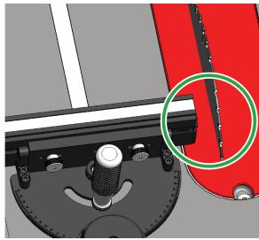
7. Adjust the Fence Assembly to the left or right as needed, then tighten the *Thumbscrews* on the back side of the Miter Gauge Body to secure the fence from moving during cutting operations.
