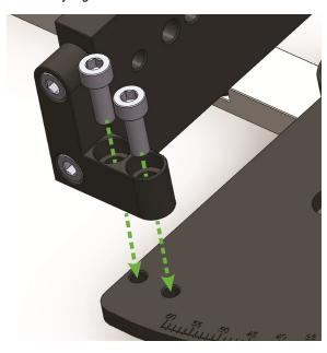
2. Note that the diameter of the holes in the L brackets are slightly oversized to provide for precise positioning (squaring) of the Vertical Faceplate with the rest of the assembly. To prepare for squaring, loosen the Grip (A) slightly by turning it counter-clockwise.
