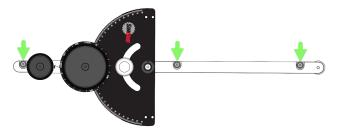
Begin with the middle adjustment disc, then adjust the front disc. Adjust the disc at the rear of the miter bar last.
