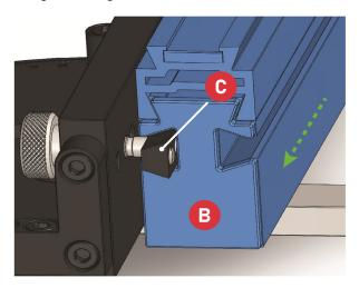
6. With the machine powered off, place the miter gauge into the miter slot of your machine. Move the miter gauge down the length of the miter slot and confirm that no part of the Fence Assembly is in the path of the blade. See additional details about USING THE FENCE SYSTEM on page 14.
