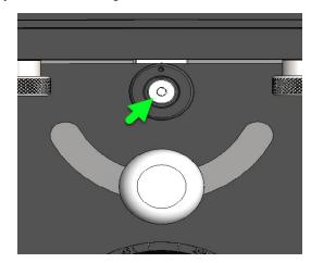
2. Rotate the adjustment bushing as needed. The gear mesh is tightest when the bushing marking is furthest from the handle (12 o'clock).
