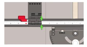
The fence extension comes into play when fixed-length cuts longer than 19.5" (49.5 cm) are required. Follow the steps below to set your flip stop and fence for this extended cut capacity.
