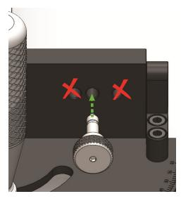
2. At the front of the *Vertical Faceplate*, loosely thread one of the *Sliding Wedges* onto the tip of the knurled *Thumbscrew*.
