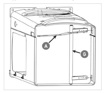
3. Place the end of the caster support (G) next to the back of the saw is the end with the mounting shoulder. Insert the mounting shoulder through the mounting hole in the rear of the cabinet and secure that end of the caster support to the cabinet with one M8 x 20 button head socket bolt (3), one M8 x 13.6 lock washer (2), and one M8 x 18 washer (4). Fully tighten the bolt using a 5 mm hex wrench.
